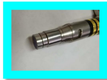
3.2 QBH homing "two points and one line" 3.3 alignment insertion of optical fiber plug
