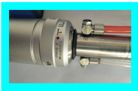
3.4 secondary locking clockwise
