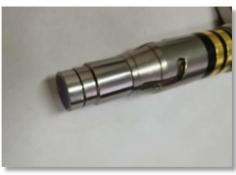
5.2 The QBH is in the unlocked position (arrow pointing to the unlocked logo) and the red dot of the fibre optic plug is inserted into place against the red dot on the end of the QBH.
