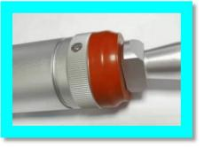
Note: The laser head needs to be placed horizontally when inserting the fiber; ensure that the fiber is inserted horizontally
