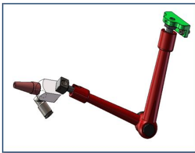
Installation diagram of universal joint side blowing
