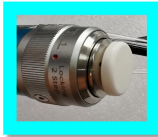
3.2 QBH homing "two points and one line" 3.3 alignment insertion of optical fiber plug
