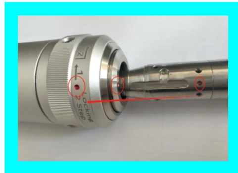
3.4 secondary locking clockwise 3.5 optical fiber protective jacket for complete protection
