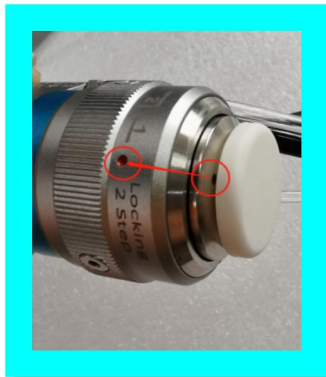
3.4 secondary locking clockwise 3.5 optical fiber protective jacket for complete protection
