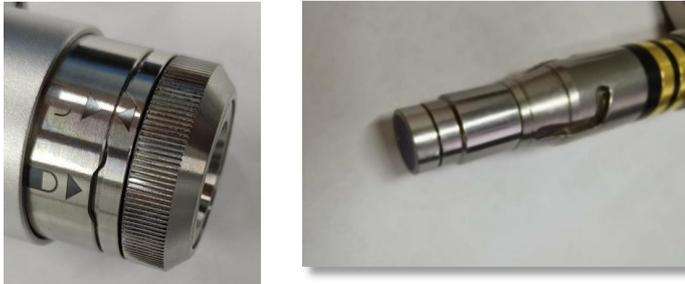
5.2 The QBH is in the unlocked position (arrow pointing to the unlocked logo) and the red dot of the fibre optic plug is inserted into place against the red dot on the end of the QBH.
