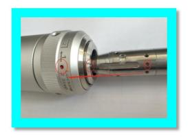
4.4 Secondary locking clockwise 4.5 Fiber optic protective jacket, fully protected
