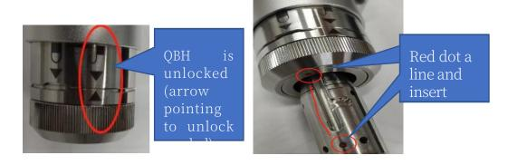
5.2 Turn the locking ring on the QBH connector clockwise until the QBH is locked (arrow pointing to the locking ring) and then tighten the locking ring.
