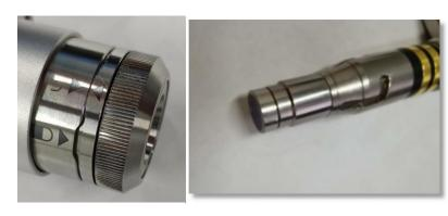
5.2 The QBH is in the unlocked state (arrow pointing to the unlocked mark) and the red dot of the fiber optic plug is inserted into place a g a i n s t the red dot on the QBH end face;
