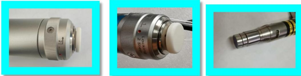
3.2 QBH homing "two points and one line" 3.3 alignment insertion of optical fiber plug
