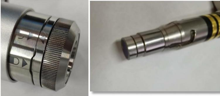
4.2 The QBH is in the unlocked position (arrow pointing to the unlocked logo) and the red dot of the fibre optic plug is inserted into place against the red dot on the end of the QBH.
